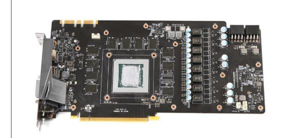
Clean up and reapply GPU core thermal grease
