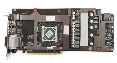
Remove the red position screw Clean up and reapply GPU core thermal grease
