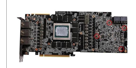
2. Remove the red position screws in the picture
