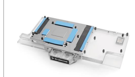
4. Stick the corresponding specifications of thermal grease in the corresponding position, paying attention to the cutting size
